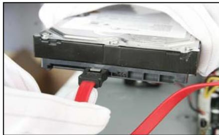
**4.** Connect the power cable to the HDD.
