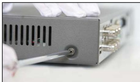
2. Install the HDD in the HDD rack using the provided screws. Fasten the screws on the button to fix the HDD.
